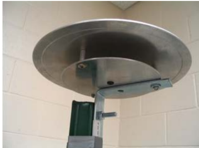
Figure 7.1 – Housing attached to L-bracket.
