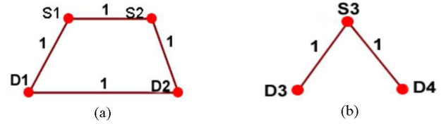
Fig. 3. (a) and (b) Two simple supply networks with supply nodes (denoted with S) and demand nodes (denoted with D). Each edge represents a distance of 1.
