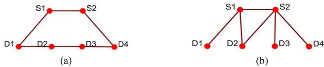
Fig. 2. (a) and (b) Two sample distribution networks with the same number of supply (S) and demand (D) nodes and edges. Network in (a) can maintain flow of supplies better than the network in (b).
